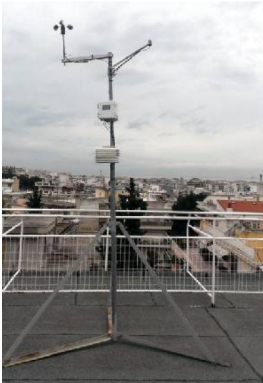
Meteorological station at rooftop.
